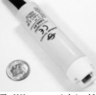
The 3203 vent-captor is designed for monitoring air flow in demanding applications. The unit operates with no moving parts and has been rated by CSA/UL to UL 1604 Class 1 Div. 2 for hazardous environments. Applications include exhaust monitoring for paint booths, air flow monitoring for factory ventilation systems and purge air/reactant air monitoring and metering for fuel cells.
