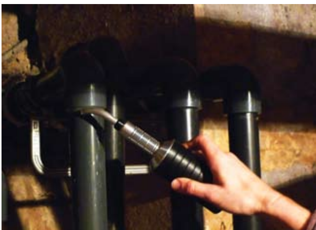
There are a slew of different leak detection and location methods. Tracer gas has proven to be particularly reliable.
